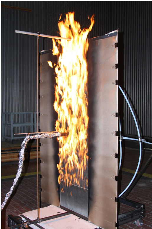
Figure 6. Photograph of ethylene wall flame experiment.
