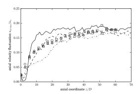
(b) Mean turbulent intensity on centerline
