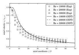
(a) Mean axial velocity on centerline
