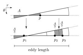
Figure 2: Illustration of particle displacement by a cylindrical triplet map
