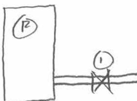
$$\rightarrow V_1^2 = 2(h_R - h_I) \\ = 2C_p(T_R - T_I)$$
